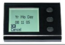
Press the middle button to scroll to and select  $\mathbf{OK}$  to save the new time setting.
