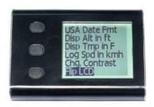
Using the **Flip LCD** function on the **Display Opt** menu, your N3 can be oriented with the buttons in either direction, on either side of your helmet.
