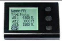
Repeat the process for the other Alarm Altitudes and once all values are set, scroll to and select **Save**. The new alarm settings are now active.
