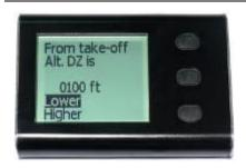
Once the target altitude is set, use the top and bottom buttons to select if the target DZ is lower or higher.
