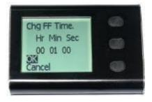
Use the top and bottom buttons to change the number of hours. Press the middle button to move on to the minutes, and so forth.
