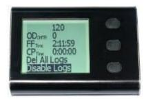
If logging is enabled, **Disable Logs** will appear at the bottom; otherwise, **Enable Logs** will appear.
