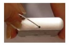
Gently insert the end of a paper clip, or similar thin utensil, press and hold the reset button for five to eight seconds.
