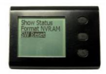
Select **SW Reset**, and then select **OK** to restart the main program. N3 will show you the **Alti-2** greeting screen, then the firmware version and unit serial number will appear. After a few seconds N3 shows the Ground Screen, and then the screen blanks. Press any button to bring the screen back into view.
